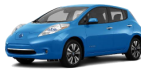
Nissan Leaf (2011-17) Electric Range = 73 mi. (2011-12) Electric Range = 75 mi. (2013) Electric Range = 84 mi. (2014-16) Electric Range = 107 mi. (2016-17)
