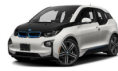
BMW i3 REx PHEV (2014-18) Electric Range = 72 mi. (2014-16) Electric Range = 97 mi. (2017-18) Total Range = 150 mi. (2014-16) Total Range = 180 mi. (2017-18)
